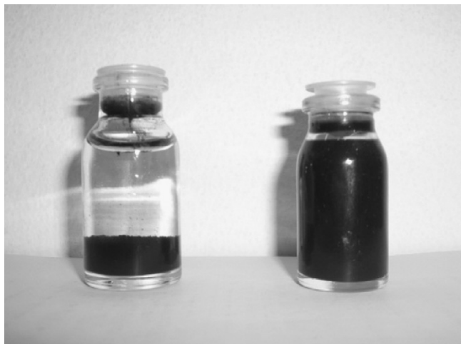
Fig. 5. Solubility photo of carbon black (left) and grafted carbon black (right) in water.
